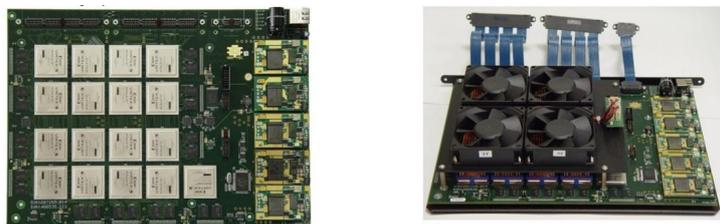
**Figure 4.** The printed circuit board of the basic module 16V5-75
