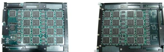
**Figure 1.** Front and back sides of the board of the RCS MPA basic module
