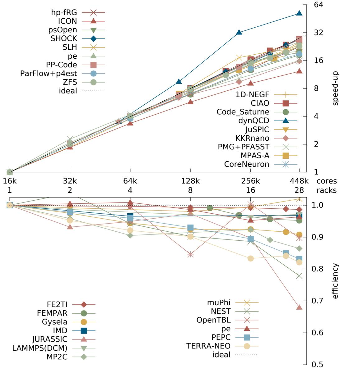
**Figure 5.** Strong and weak scaling of High-Q Club member application codes on *JUQUEEN*. Compared to a single rack, ideal strong scaling has a speed-up of 28 $\times$  on 28 racks and weak scaling has 100% efficiency. Of the 18 codes showing strong scalability, ten maintained scaling efficiency above 80%, and only three were below 65% efficiency
