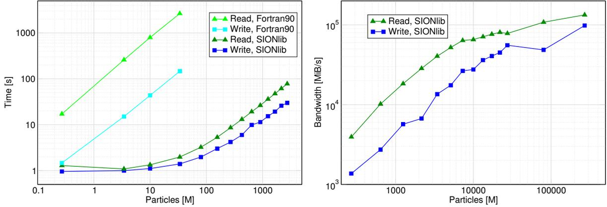
**Figure 6.** Left: MP2C file I/O time on one *JUQUEEN* midplane (8,192 MPI ranks) using traditional F90 I/O compared to improved I/O with *SIONlib*. Right: MP2C file I/O bandwidth for checkpointing executions with 1.8 million MPI ranks on 28 racks of *JUQUEEN* using *SIONlib* for reading and writing particle data
