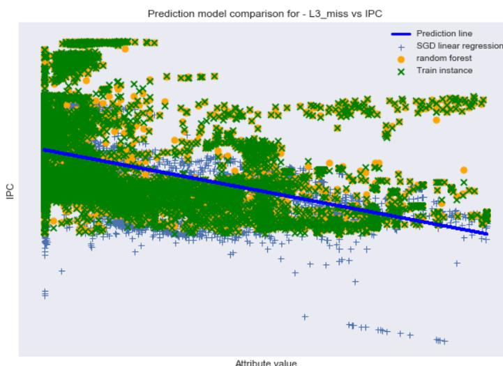
**Figure 8.** Scatter plot of L3 miss rate vs IPC from the training data set. Also plotted are the predictions based on the single-attribute linear regression, the multi-attribute SGD linear regression, and the random forest
