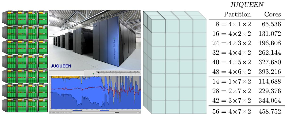
**Figure 1.** *JUQUEEN* Blue Gene/Q as presented by the *LLview* system monitor (28 racks with two midplanes each with 16 nodeboards of 32 processors), schematic of the 56 BG/Q rack midplanes arranged  $4 \times 7 \times 2$  and list of partitions with corresponding number of cores available when scaling rows or columns of racks to the entire configuration
