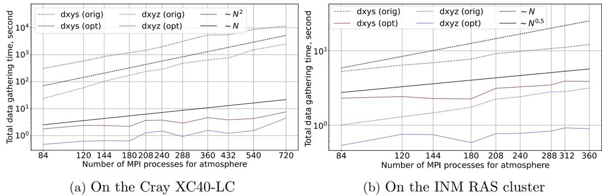
**Figure 6.** INMCM6M optimized 3D output gathering time against the number of MPI processes for the atmosphere component
