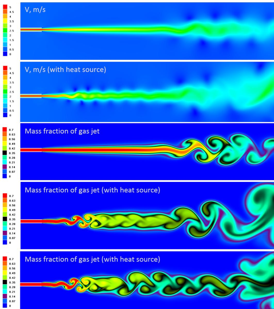
**Figure 6.** Results of simulation of jet instability at velocity  $V = 5$  m/s for case without and with excitation of a jet by a heat source with a frequency of 500 Hz. Bottom image shows a temporary change in the flow structure caused by an increase in energy input
