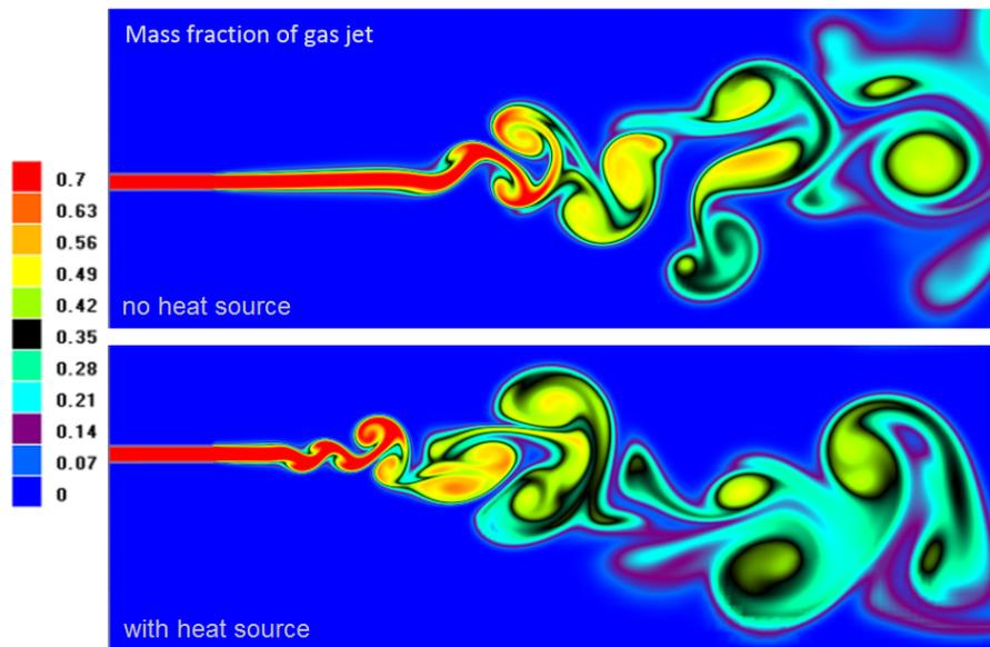
**Figure 8.** Visualization of a jet without a discharge and with a discharge simulated by heat source. Results of simulation at velocity  $V = 10$  m/s
