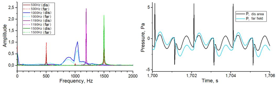
**Figure 4.** Spectra of pressure fluctuations in the jet with varying frequency of exposure and Pressure pulsations caused by a periodic heat source with a frequency of 1500 Hz
