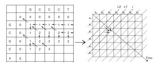
Figure 3. Parallel Constructing Smith-Waterman Matrixalong Diagonal
